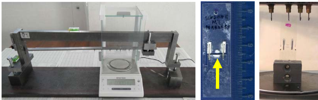
Figure 3. On the left, photo of the new micro-cycling machine. On the middle, the special polyester mask in which the flax fiber is clamped (evidenced by the arrow). On the right the tabbed fiber clamped on two iron masses and leaned on the plate of the analytical balance after having broken the two lateral strips using an iron wire as heating source.
